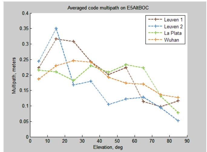
**Figure 22. Code multipath on E5AltBOC at 4 locations. Here Leuven-1 is our main open-sky antenna site (Figure 2). Leuven-2 is more multipath-rich site located between the ventilation outlets (see previous section)**
