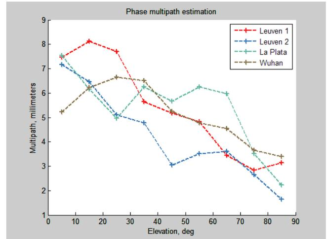
**Figure 31. Phase multipath at 4 locations. Here Leuven-1 is our main open-sky antenna site (Figure 2). Leuven-2 is a more multipath-rich site located between the ventilation outlets (see previous section)**
