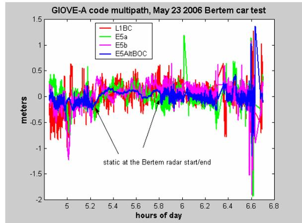
Figure 28. Code multipath during the rural car test.
