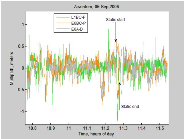
**Figure 30. Code multipath during the urban test.**
