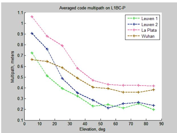
**Figure 21. Code multipath on L1BC at 4 locations. Here Leuven-1 an open-sky antenna site (Figure 2). Leuven-2 is more multipath-rich site located between the ventilation outlets (see previous section)**
