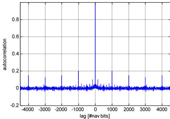
**Figure 2. Autocorrelation of the L2P navigation bit stream.**
