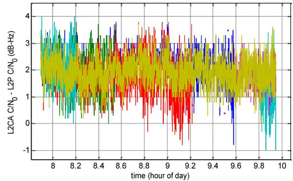
**Figure 4. Carrier-to-noise ratio difference between L2CA and L2P.**
