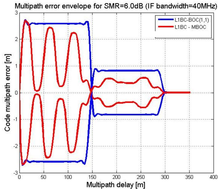
**Figure 2. Multipath error envelopes of MBOC versus BOC(1,1) computed at a signal/multipath ratio of 6 dB.**
