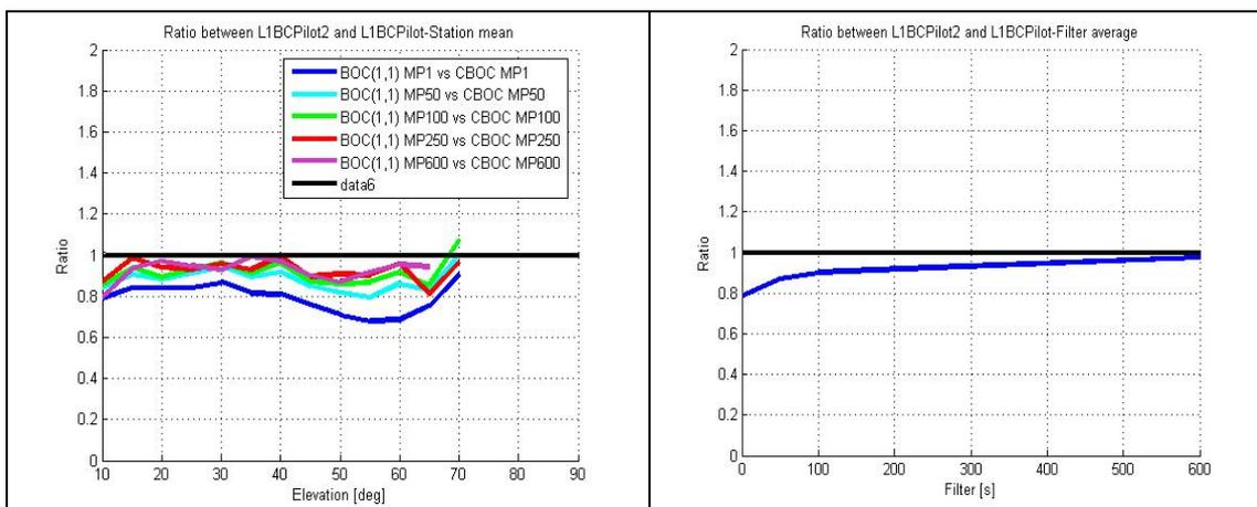
**Figure 7. Left side: ratio of the range error STD ratio of CBOC/BOC(1,1) as a function of the elevation angle for various filtering windows (1,50,100,250, 600s ). Right side: total standard deviation as a function of the filtering window.**
