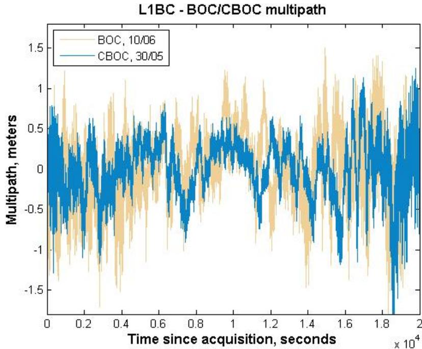
Figure 5. Multipath time series for L1BC for May 23, when BOC(1,1) was transmitted, are compared to June 10, when CBOC was transmitted (comparison by method (a)).
