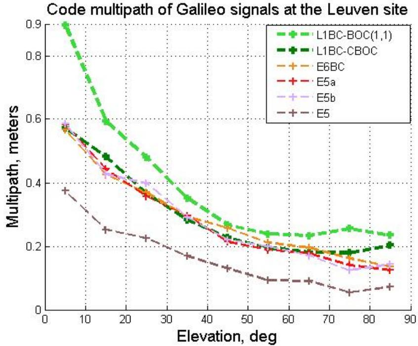
Figure 4. STD of code multipath for Galileo signals transmitted by GIOVE-B. The two thicker lines indicate L1BC modulations: BOC(1,1) and CBOC.
