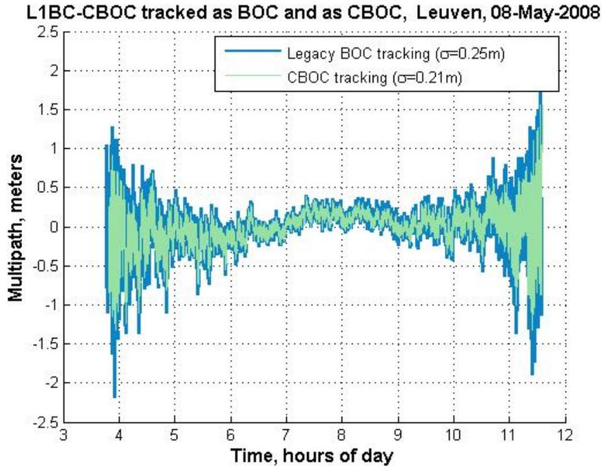
**Figure 6. Simultaneous multipath time series of BOC(1,1) (blue) and CBOC (green) obtained by the tracking of CBOC in two modes (comparison method (b)).**
