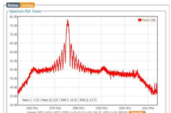
**FIGURE 1:** The spoofed GPS signal from a HackRF SDR shown in the spectrum plot of the [AsteRx-m2a](#) Web Interface. The SDR reproduces the sinc shape of the BPSK signal modulation with a power which in this case, is about 25 dB higher than the real signal.
