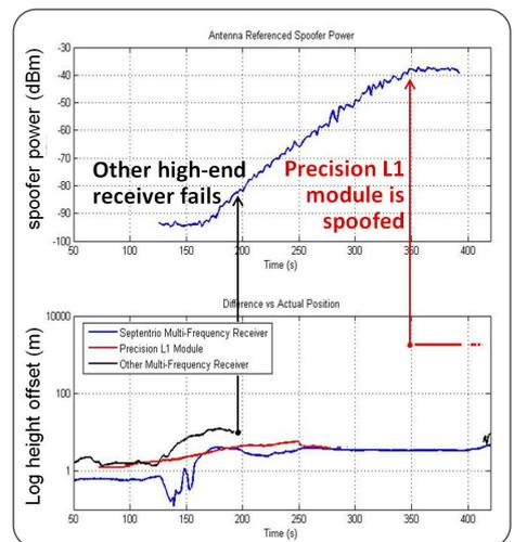
**FIGURE 4:** Height plot comparison for three different receivers subject to spoofing as the spoofer power is increased. The Septentrio AsteRx4 position survives to maximum spoofer power thanks to frequency diversity.
