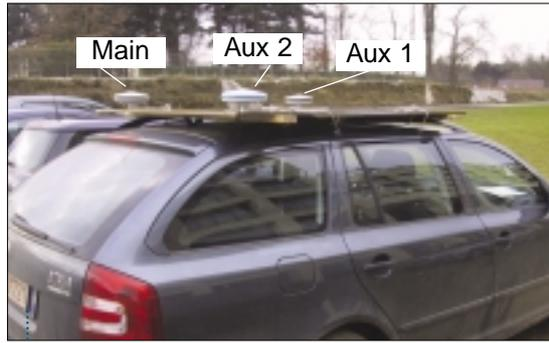
Figure 4 - Antenna installation on car.
