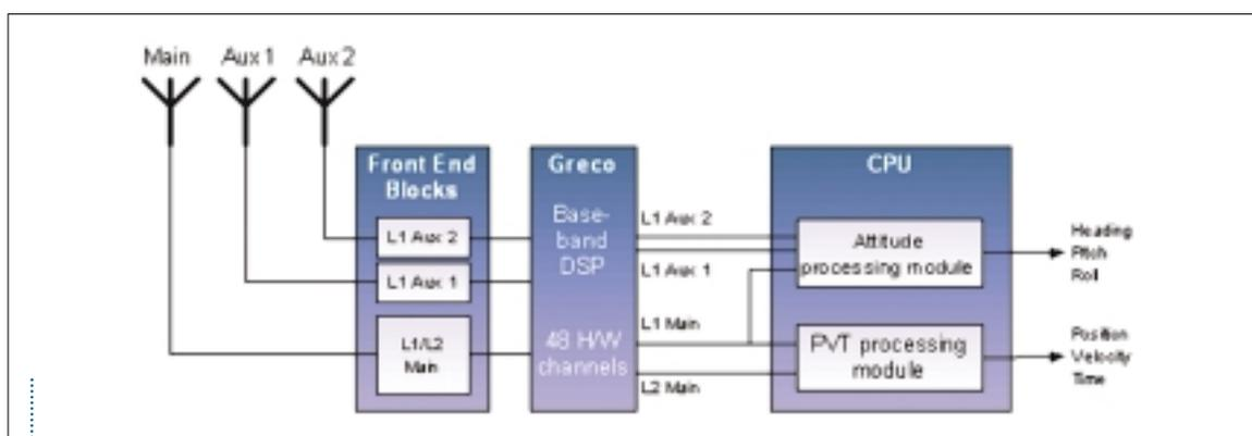
Figure 1 - Single-board triple-antenna PolaRx2@ GPS receiver.
