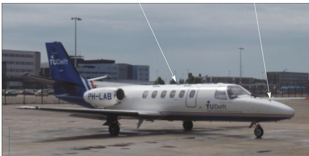
Figure 6 - Antenna setup Cessna Citation II (Delft University of Technology).
