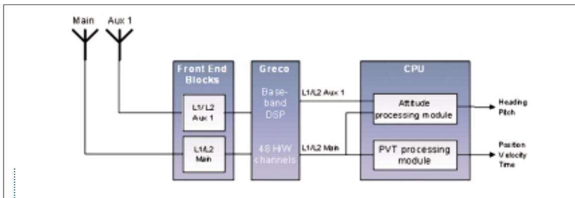
Figure 2 - Single-board dual-antenna PolaRx2HD GPS receiver.
