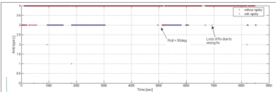
Figure 8 - Fix characteristics during flight (4: fixed, 3: float).
