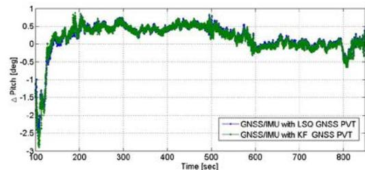
**Figure 6 Pitch error, using PolaRx2eH reference**
