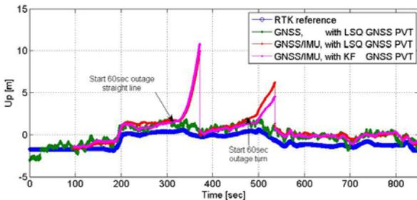
**Figure 12 Vertical trajectory with 60 sec outages**
