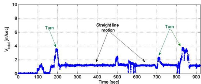
**Figure 5 Total velocity during combine harvester operation**
