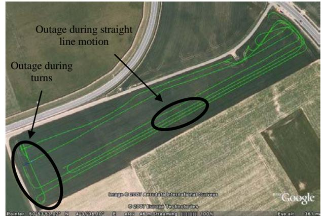
**Figure 2 Test environment and trajectory – Steenokkerzeel (Belgium) ©Google**
