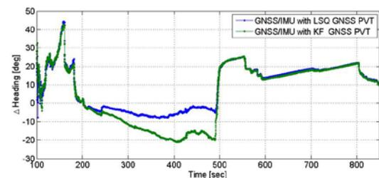
**Figure 7 Heading error, using PolaRx2eH reference**
